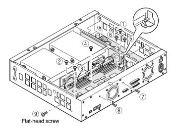
6. Connect the cables to the RAID board.
