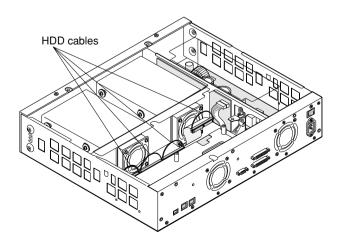
3. Connect between the main and RAID boards with 2 cables that belong to the main board.
