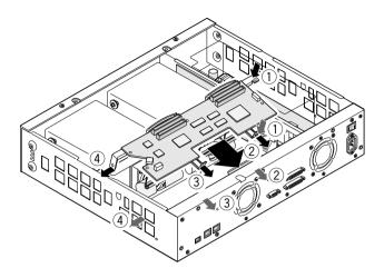
(2) Secure the RAID board to the main unit with the screws (6 screws with washer for top of the board, 2 screws for rear of WJ-ND300, and 1 flat-head screw for side of WJ-ND300) attached to the board.
