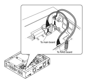
4. Detach the cable from the cable clamp to unbind it, and pass the cable through the cable clamp as shown in the illustration below.
